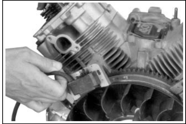
Figure 11-49. Installing Ignition Module.
